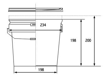
Measurements in millimetres
